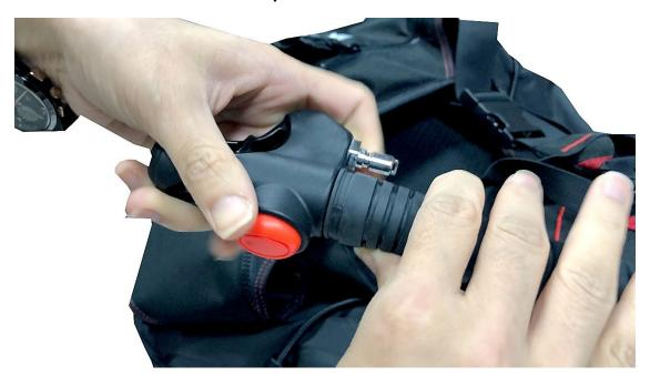
2-3. If there is a pull-dump wire connected, use a sharp cone to push and remove the pin on the inflator and disconnect the wire.
