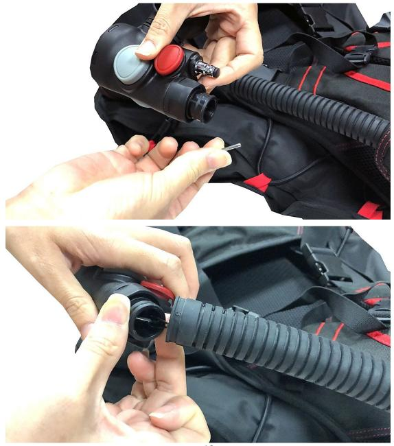
3-2. Assemble the IF-O with the corrugated rubber hose of the BCD and secure with a zip tie.
