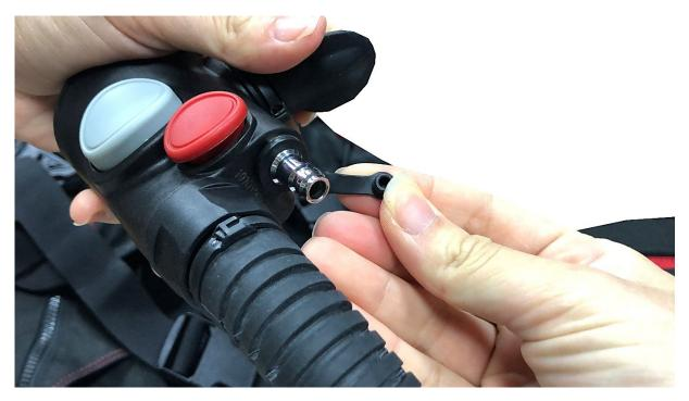
3-5. Connect the IF-O to the regulator with a low-pressure BC hose.
